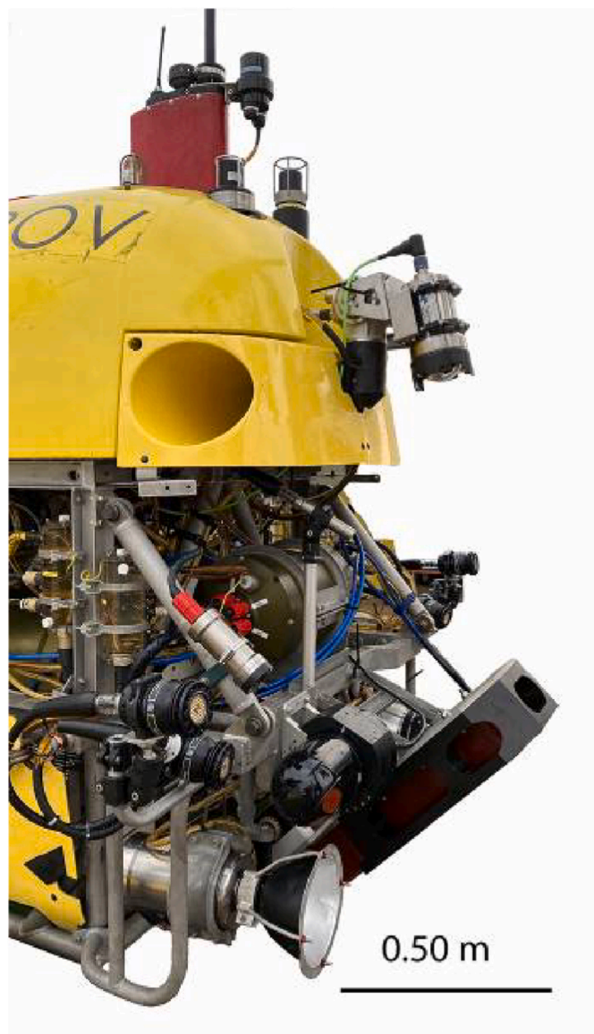
Fig. 1. Image of Ariane H-ROV with the Kongsberg EM2040 Multibeam Echosounder installed with a 45° angle.
